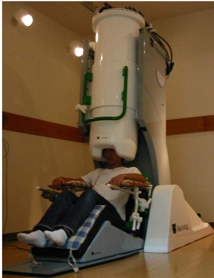
Photo 1. 122-channel whole-head neuromagnetometer (Neuromag-122™, Neuromag Ltd., Finland)
