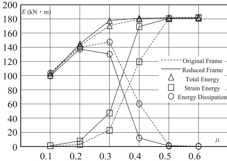
**Figure 6.** Relationship between coefficient of friction and energy
