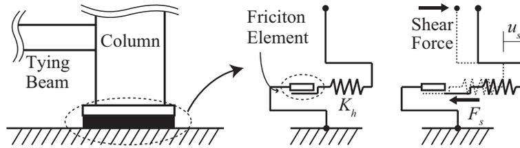
**Figure 2.** Analytical and mechanical models of friction damper
