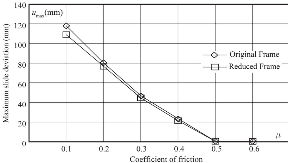
Figure 5. Relationship between coefficient of friction and maximum slide deviation
