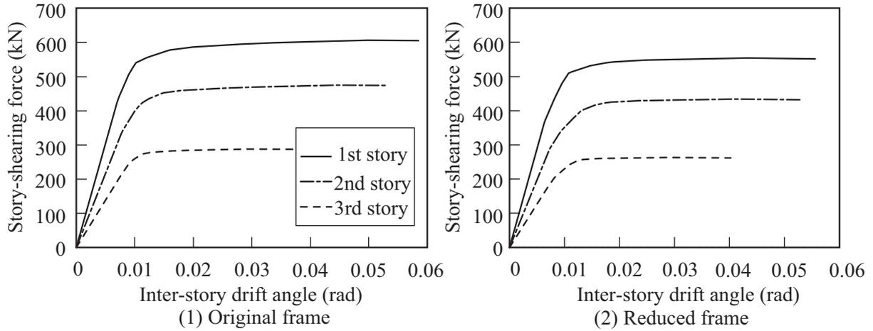
**Figure 3.** Relationship between shear force and inter-story drift angle
