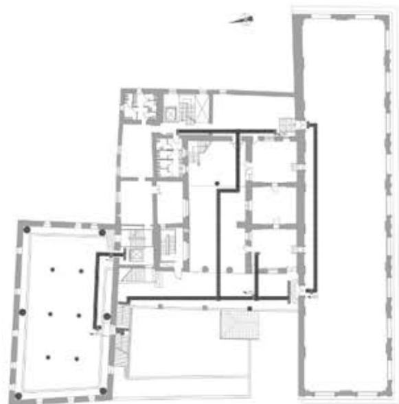
Figure 15: Second floor: the LOGES system.
